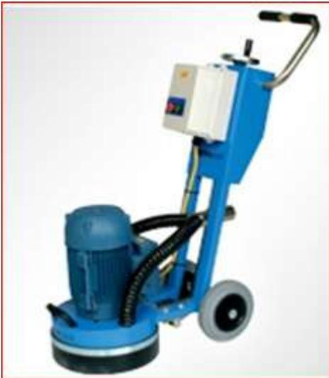
A Typical Small Floor Grinding Machine
